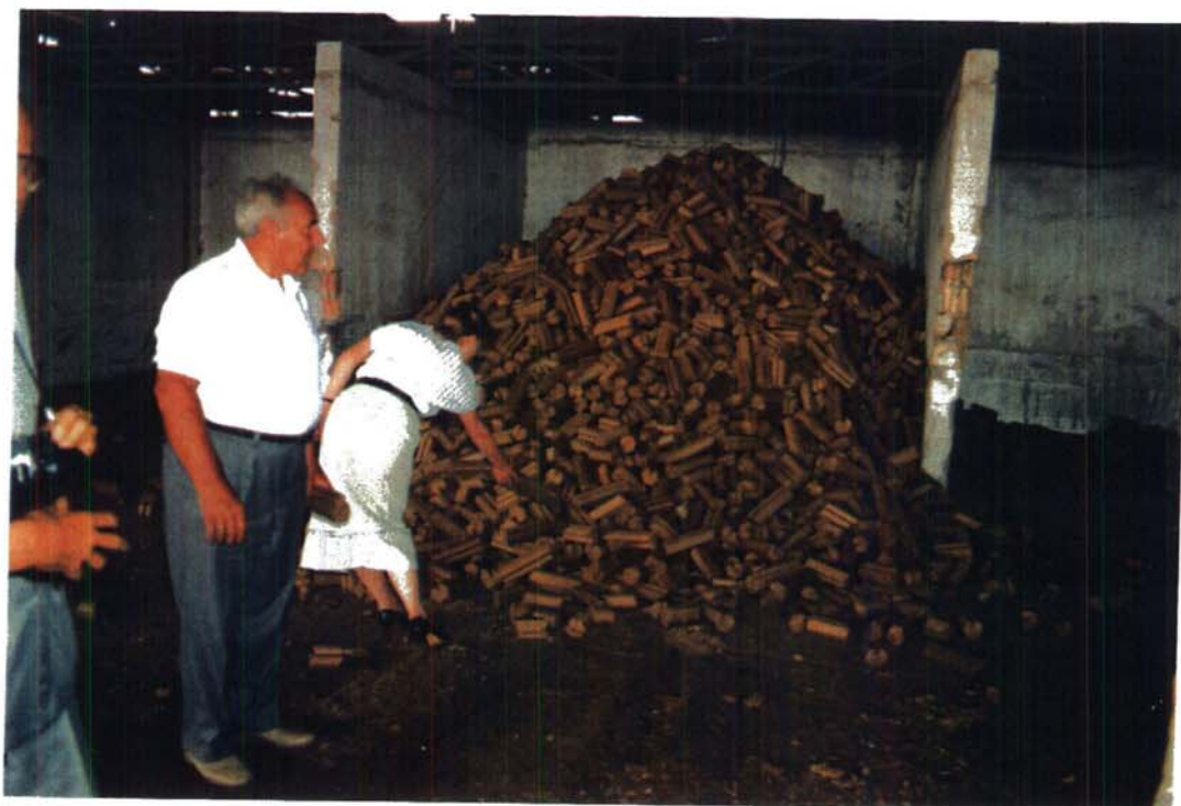
Plate 8: Straw briquettes produced from the light straw fraction at Dunaujvaros Paper Mill, Hungary
